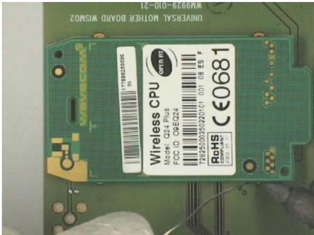
Turn the application board and solder the 4 legs on this side.
