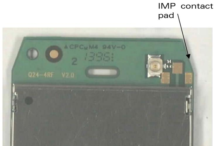
Figure 13: Assembly process - IMP connector
