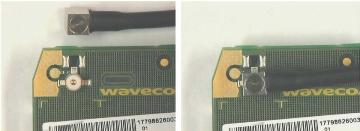
Figure 6: Assembly process - MMS connector
