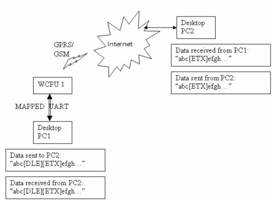
The above schematic explains how [ETX] characters - which have a special meaning in WIP soft – are handled on Wavecom Wireless CPU<sup>®</sup>.
