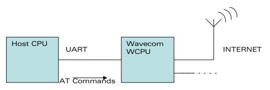
Multiplexing: Several sockets can be operating at once. The +WIPDATA command allows to temporarily identify the UART in data mode with a given socket. The data written on UART is transferred through the socket. The data which arrives on the socket can be read from the UART.
