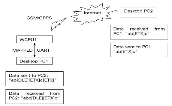
The above schematic explains how [ETX] characters which have a special meaning in WIP soft are handled on Wavecom Wireless CPU<sup>®</sup>.
