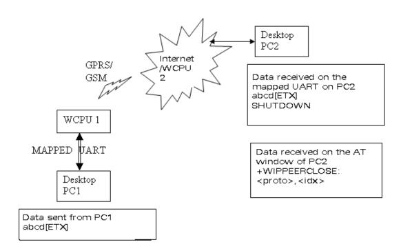
In the above schematic, a TCP socket is connected. On the transmitting side, data and [ETX] is sent (use case: Desktop PC1 is a Wireless CPU<sup>®</sup> which sends data to PC2 which is either a PC or a Wireless CPU<sup>®</sup>), the data is received on PC2 and [ETX] character shutdowns the socket on the transmitting side and displays a message "[CR][LF]SHUTDOWN[CR][LF]" on the mapped UART of PC2.
