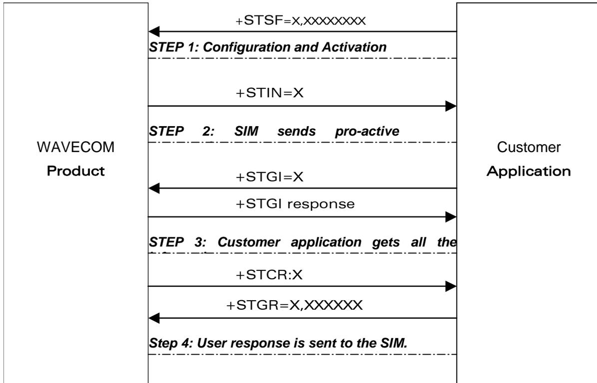
On the first step, the customer application informs the Wavecom product which facilities are supported. This operation is performed with the **+STSF** (*SIM ToolKit Set Facilities*) command, which also allows to activate or deactivate the SIM Toolkit functionality.
